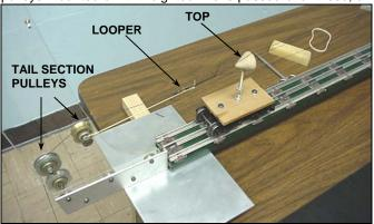
applies tension to the looper and carriage. The size of the rope being formed will determine how much weight is utilized. When working with fine thread, tension on the carriage may not be needed at all. Filipowski suggested keeping a log that lists what weight combinations go best with various size lines. Once you have that information, and the resultant diameters, an inventory of sizes can be made for your model when it is time to rig.
