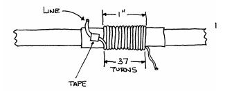
As stated earlier, the distances normally utilized are 1" and ½". When measuring extremely fine thread, covering one inch can take well over one hundred turns. If you decide to use the lesser length, it merely becomes a matter of dividing the turn count into .5 rather than 1.
