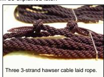
in different manners. Putting three strands on each whirl, and running them simultaneously formed one example, while the second sample was composed of three individual 3-strand hawsers, which had been twisted together.
