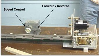
The carriage, which carries the top, is mounted on a chassis scrounged from an old model railroad caboose. It is essential that the wheels turn as freely as possible so as not to impede movement as the rope begins to form. You might want to consider making different tops for different diameter rope. The nine and twelve strand cables can get quite large!
