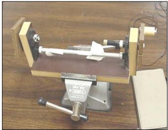
turns, which results in a decimal that represents the line size. Bob stated that just about any round object would work with this method. Some of the most common devices used are pencils, doll rod, and brass tubing.
